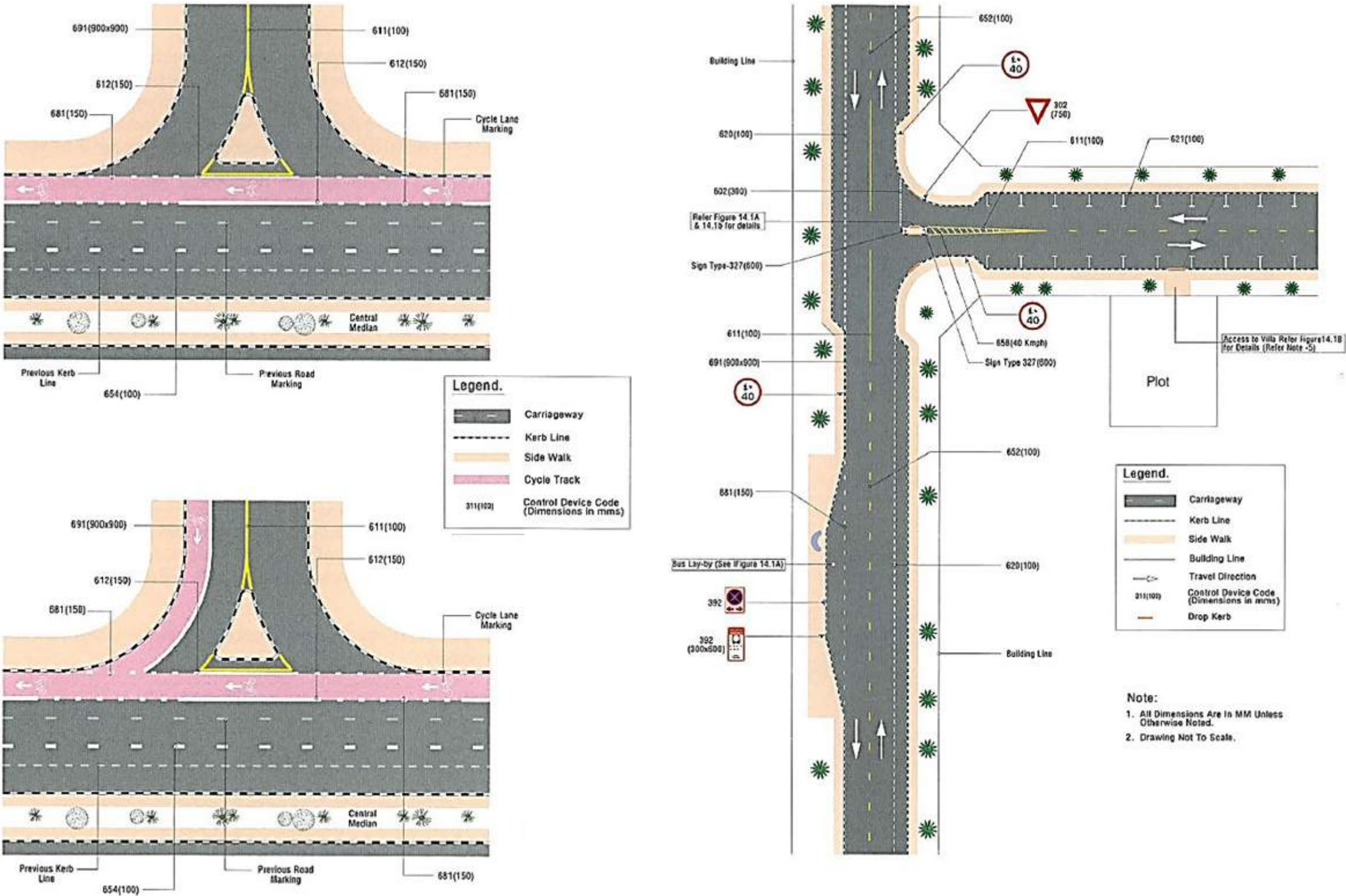
Figure 5.13 Typical Slip Road and RIRO Design Source: Dubai Pedestrian and Cyclist Design Manual, January 2006, Chapter 14
