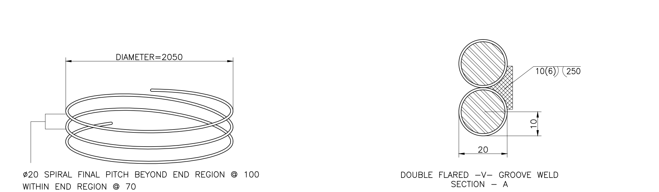
8 DETAILS OF TIES REINFORCEMENT LAP-WELD CONNECTION SCALE NTS
